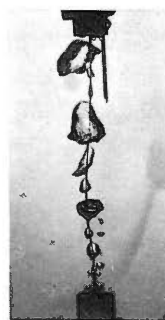
過冷度 5^\circ\text{C} q = 24.1 \times 10^4 (\text{kcal/m}^2\text{h}) (膜沸騰)
